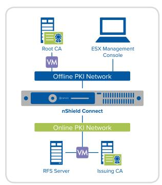
Figure 7: Leveraging nShield Connect for Offline and Online CA Virtualization
