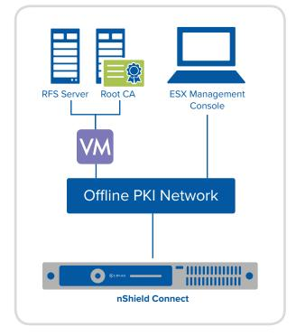
Figure 6: nShield Connect for Offline CA Virtualization
